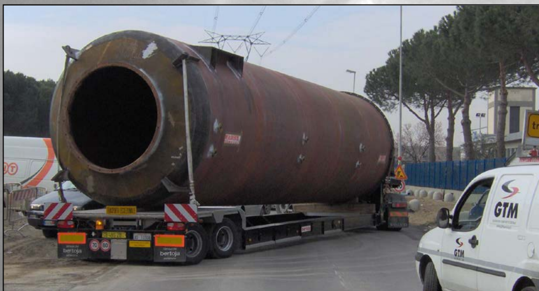
Combustore Ø3.200xHf18.000 Sp. 15mm Combustion plant Ø3.200xHf18.000 Thickness 15mm
