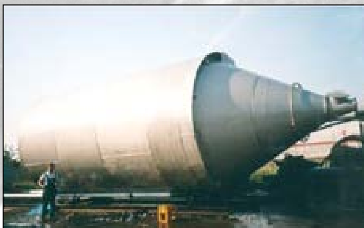
Silos per soda Inox AISI 316L Ø3.500 Sp. 15mm Silos for soda in stainless steel EN 1.4404 Ø3.500 Thickness 15mm
